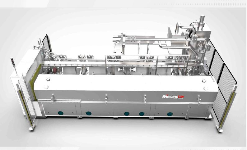
Horizontal chamber with a useful dimension of 6000 x 800 mm, able to accommodate tubes up to 6 metres long
