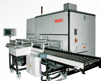
Installation standard SOLVACS 2 (dimensions des charges 530 x 320 x 200 mm)
